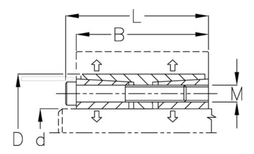
$\begin{array}{lll} \text{B mm} & = 66 \\ \text{d H8 mm} & = 50 \\ \text{D mm} & = 80 \\ \text{Fit tolerance} & = \text{Aksel h8, Nav H8} \\ \text{F kN torque} & = 87.7 \\ \text{L mm} & = 74 \\ \text{M mm} & = \text{M8} \\ \text{P N/mm2 surface pressure on shaft/hub} = 32 \\ \end{array}$
